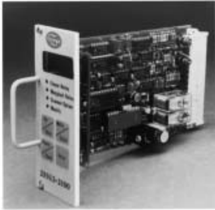
AMPLIFIER WITH KEYPAD/DISPLAY PART NUMBER 25SU3-2100
